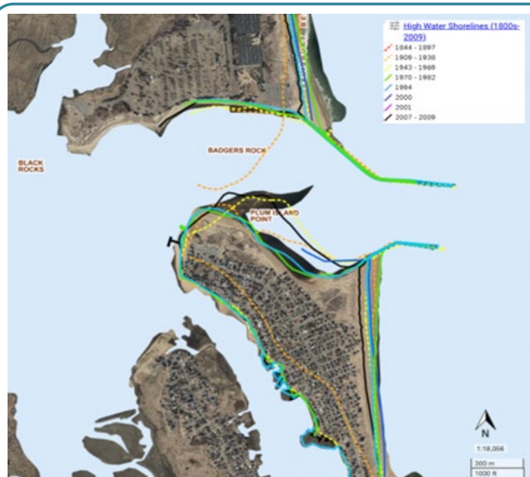
Figure 4.4 Map of the north and south jetties at the mouth of the Merrimack River with historic coastal edge data from 1909-2009. Source: Coastal Zone Management Massachusetts Shoreline Change Project.
