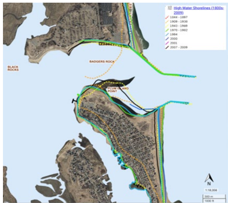
Figure 4.3 Map of the north and south jetties at the mouth of the Merrimack River with historic coastal edge data from 1909-2009. Source: Coastal Zone Management Massachusetts Shoreline Change Project.
