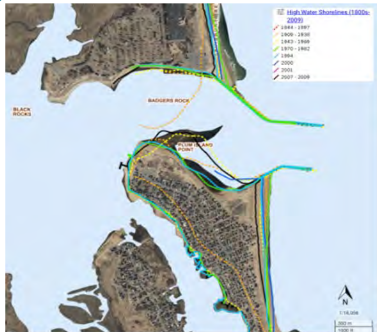
Figure 4.4 Map of the north and south jetties at the mouth of the Merrimack River with historic coastal edge data from 1909-2009. Source: Coastal Zone Management Massachusetts Shoreline Change Project.
