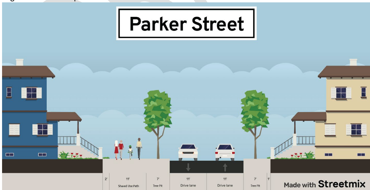
Figure 56. Illustration of Typical Cross Section for Parker Street Sidepath.
