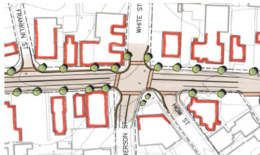
Part of the preliminary Winter Street designs, showing expanded crosswalks and new trees.
