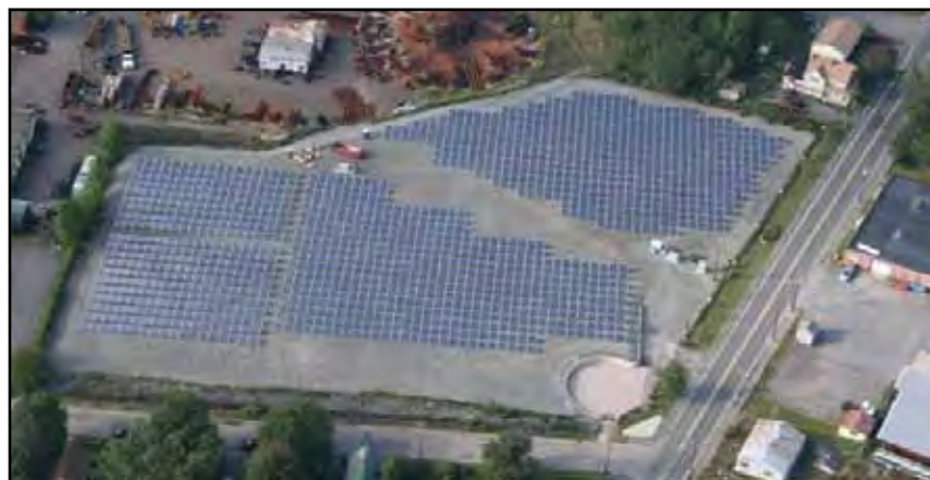
Brockton Brightfield consists of 1,395 SCHOTT Solar modules manufactured in Billerica
